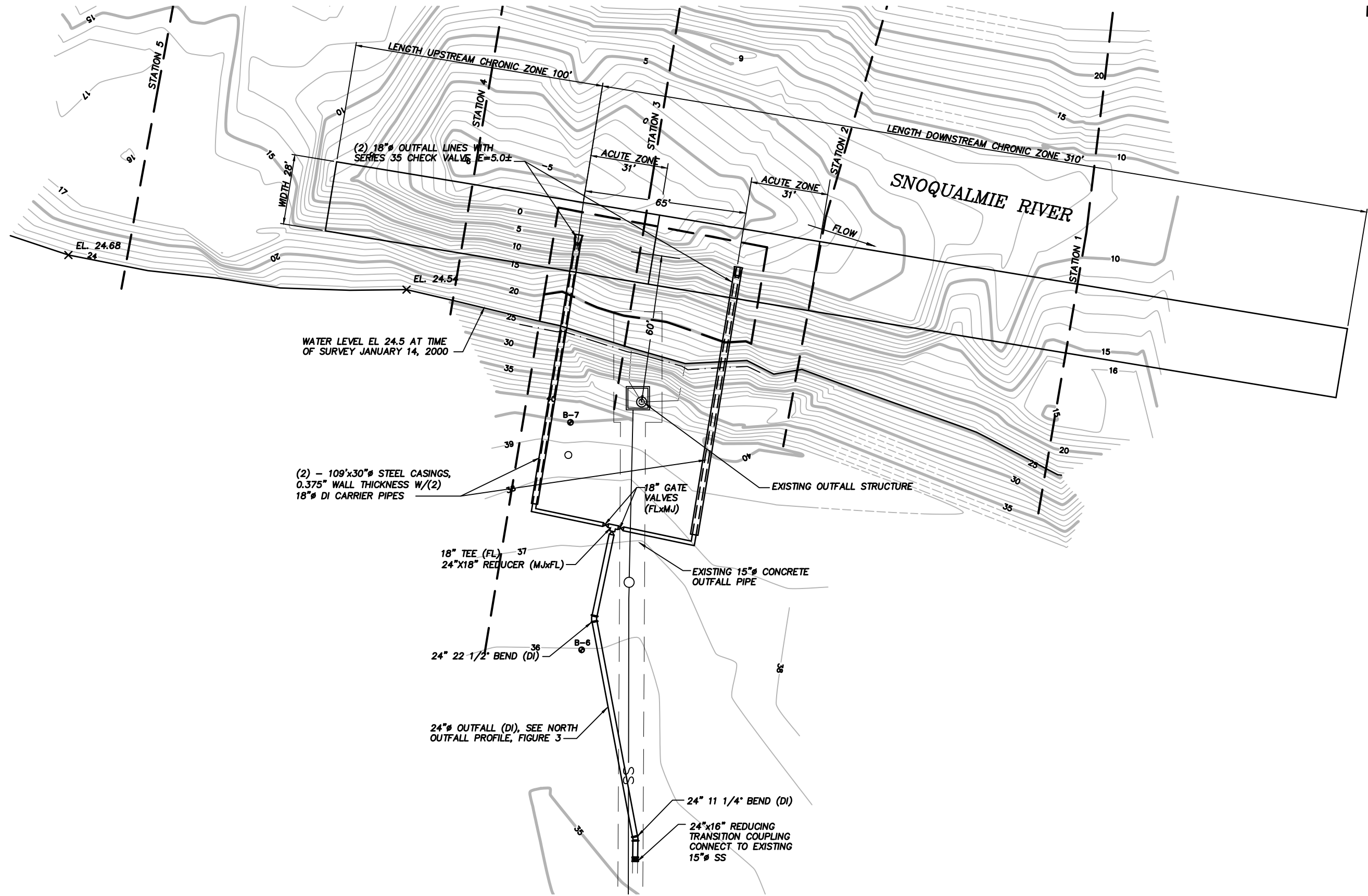
Figure 5-1 Proposed Two Port Outfall Configuration and Mixing Zone Sizes
